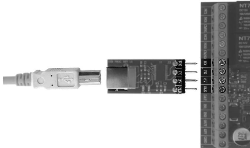
*Fig. 3.3 – USB Programmer board connection*
