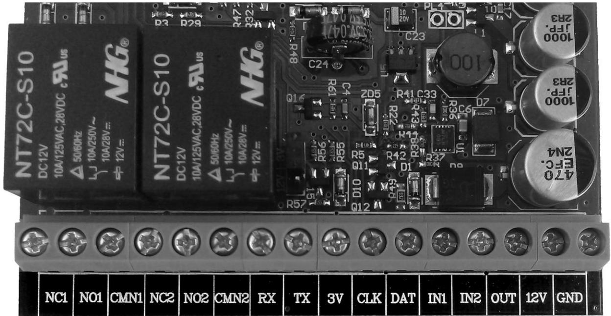
Fig. 3.1 – GSM Communicator connection terminals
